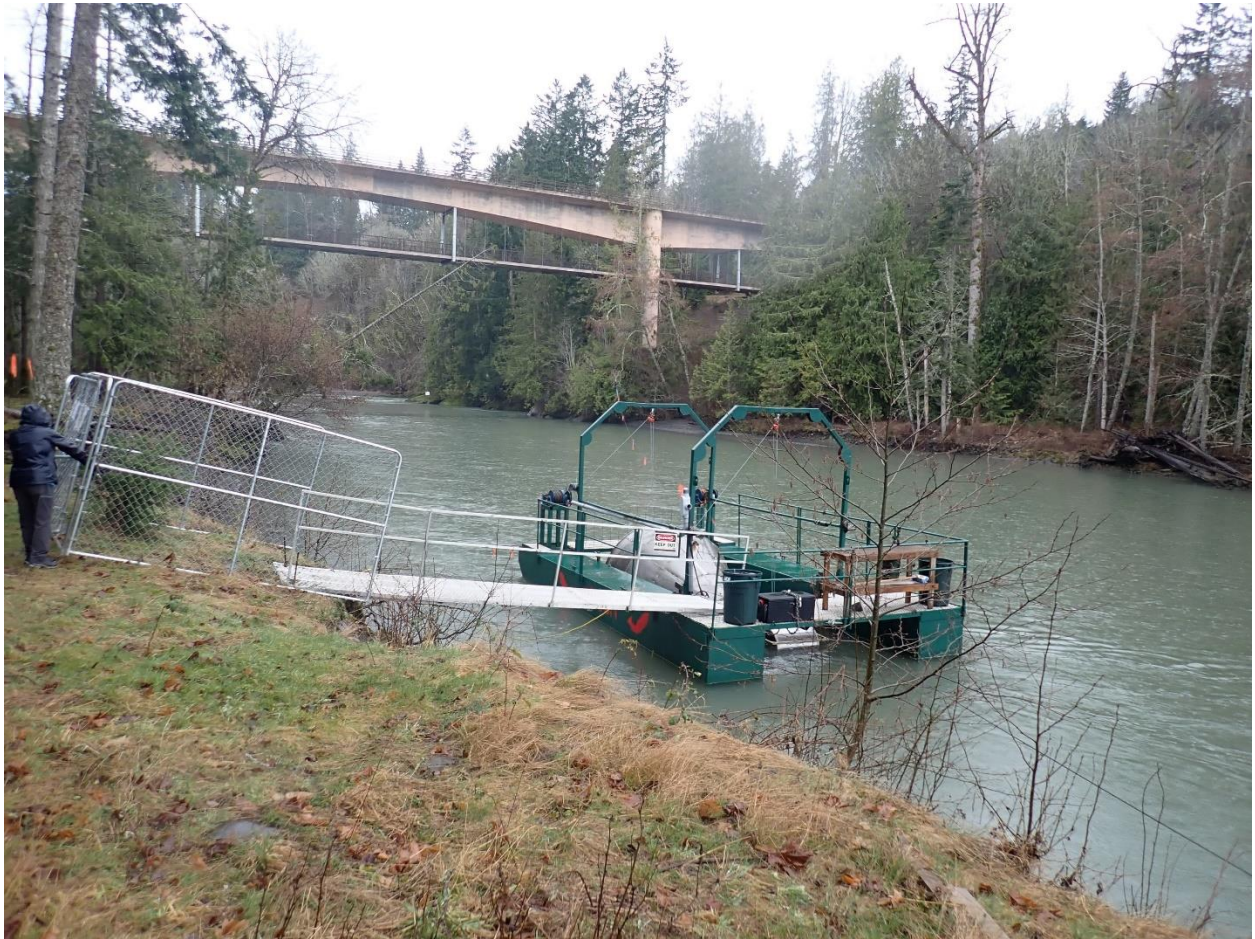
Figure 1. Top Elwha River 8' rotary screw trap fishing at Rkm 4.0 during the post-project period.
